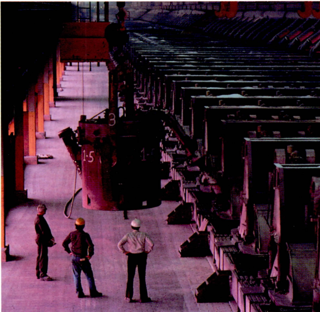
In these Hall-Heroult cells cryolite is heated to a temperature of 900 to 1,000° C.
