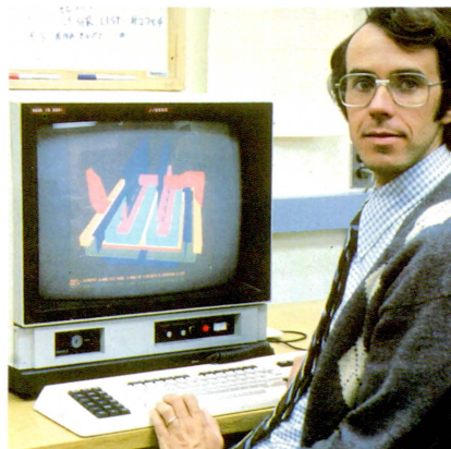
Dr. Don Ziegler shows a PATRAN rendering of a Hall-Heroult cell magnetics model on an Apollo workstation.
